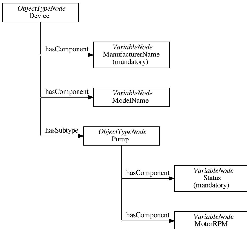
Children that are marked mandatory are automatically instantiated together with the parent object. This is indicated by a *hasModellingRule* reference to an object that represents the *mandatory* modelling rule.
