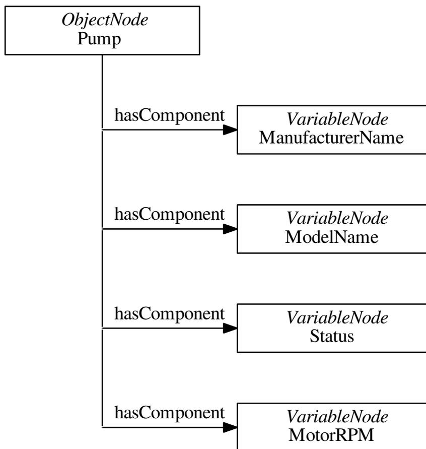
The following code manually defines a pump and its member variables. We omit setting constraints on the variable values as this is not the focus of this tutorial and was already covered.
