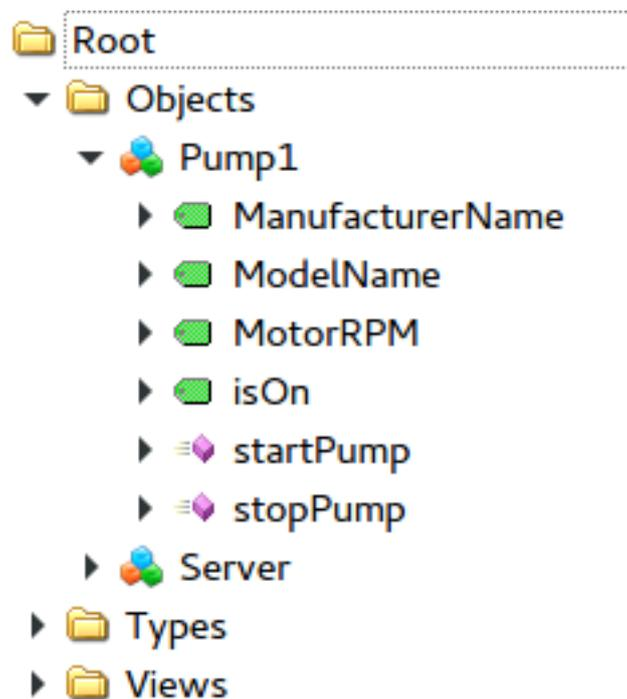
Fig. 11.1: Instantiated Pump Object with inherited children
